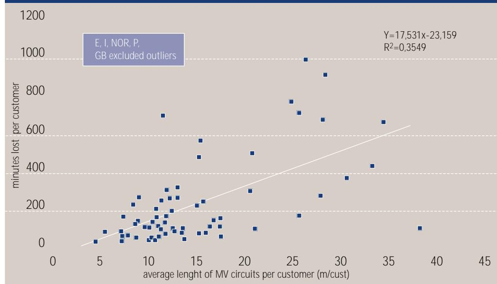
FIG. 2.11 NUMBER OF INTERRUPTIONS AND DENSITY (AVERAGE LENGTH OF MV CIRCUITS PER CUSTOMER) USING UNPLANNED INTERRUPTIONS REGIONAL DATA (2001)
