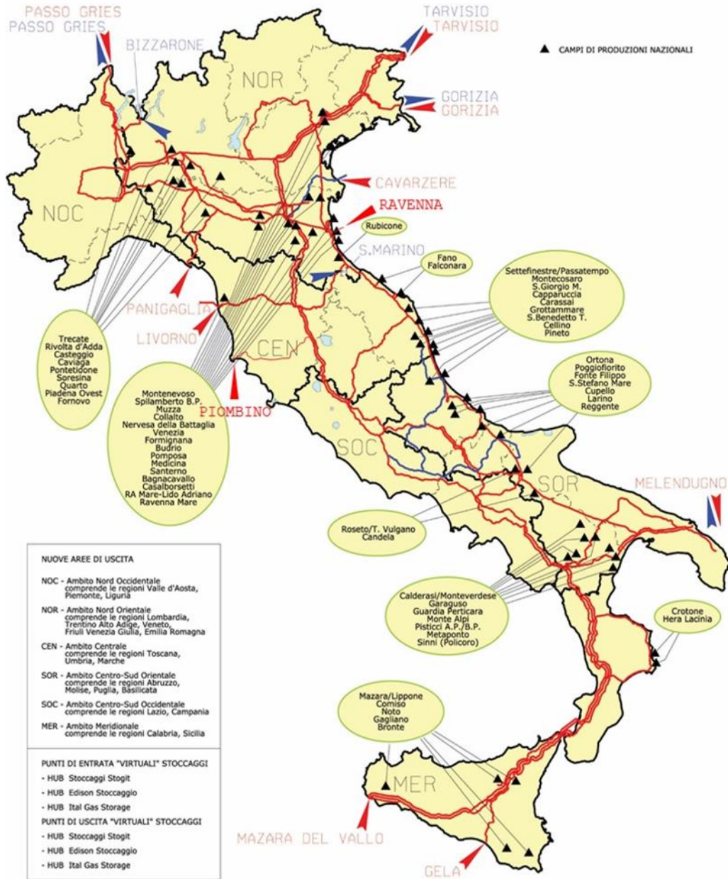
Figure 2: Representation of the network of natural gas pipelines to the year 2024 – Detail of national production
